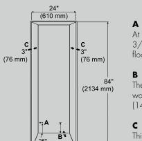
At this point the power cord exits from the appliance rear. 3/4" (19 mm) from the left and 5" (127 mm) from the floor. Free length of the power cord is 98" (2.5 m).
