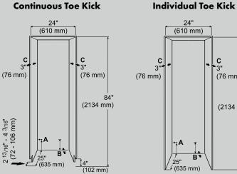
At this point the power cord exits from the appliance rear. 3/4" (19 mm) from the left and 5" (127 mm) from the floor. Free length of the power cord is 98" (2.5 m).
